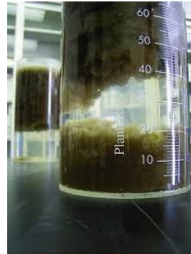
POOR Settling Sludge blanket split, DENITRIFICATION
