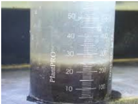
Good Settling Dense blanket, clear supernate
