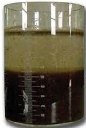
Medium Settling Uniform blanket, PIN-FLOC
