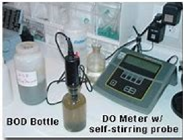
Dissolved Oxygen Uptake (DOUR) Test
