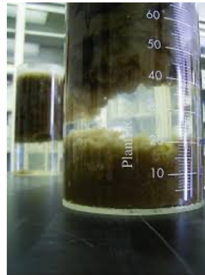
POOR Settling Sludge blanket split, DENITRIFICATION or ANNOXIC
