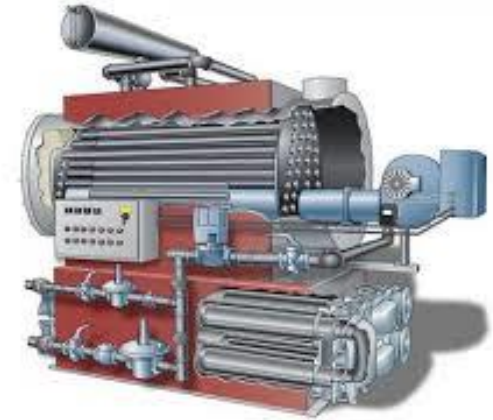
Boilers for digester heating
