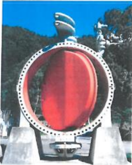
A large butterfly valve shown as partially open
